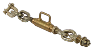
A-159350 Check Chain Stabilizer Fits most compact tractors 15 HP to 40 HP. Adjustable: 11.750" - 13.500" Body Length: 3.500" Pin Diameter: 7/16" Thread: M14-1.5
