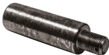
A-8013 Coulter Spindle Used To Repair Spindle On Coulter Arm. Instead Of Changing Arm, Cut Out Old Bearing Shaft, Install New Bearing Shaft And Weld In Place 3/4" Thread
