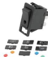
A-VLC2531 Switch, Rocker; 20 Amp, 3 Terminal, On/Off (Illuminated) Terminals: 3 Volt/Amperage: 12/20 4 Color Discs & Various Symbols For Universal Applications Fitted w/ 12 Volt Bulb Requires 1.524" X .728" mounting hole and panel .150" thick
